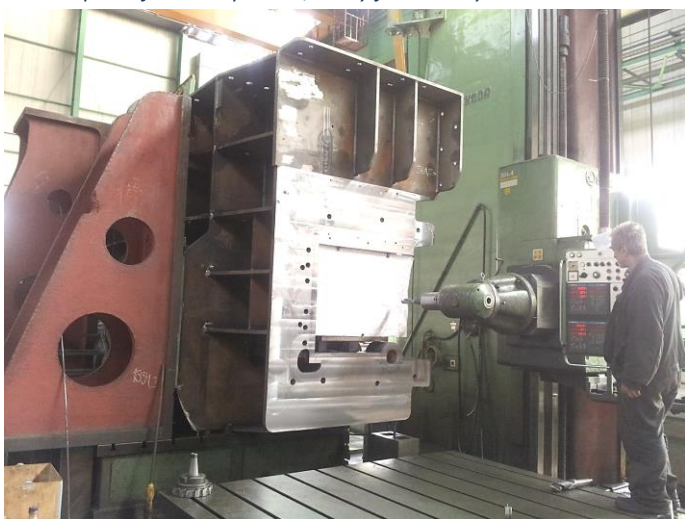
Machining of the bottom part of the scrap shear
