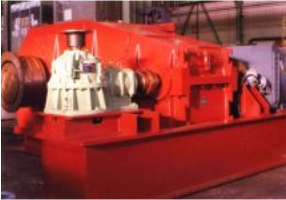
Gearbox for crane
