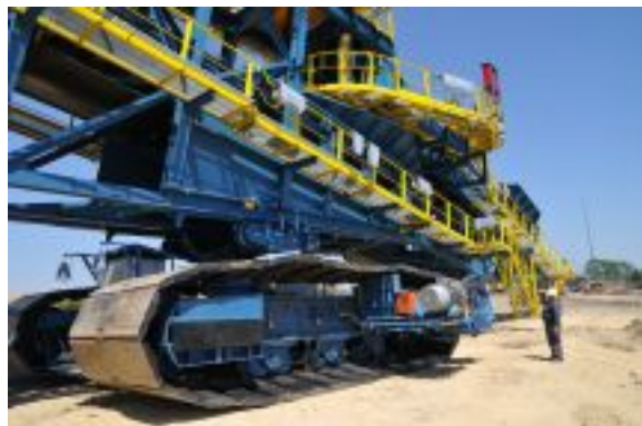
Spreader ARS2000, detail: crawler
