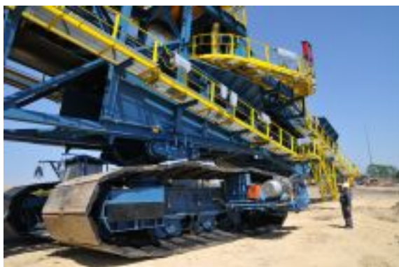
Spreader ARS2000, detail: crawler
