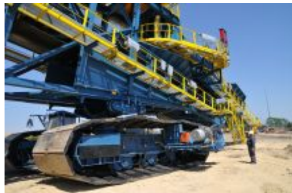
Spreader ARS2000, detail: crawler
