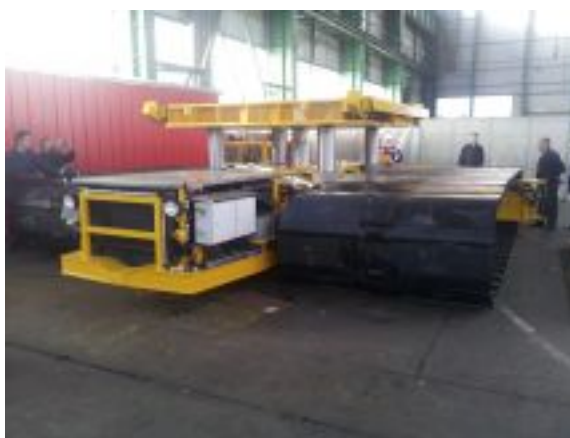
Transport crawler T300, complete production and assembly, ordered by TKF (2012)
